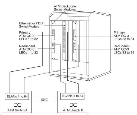
Figure 1-6 Example Dual-Homing/Module Redundancy Configuration
